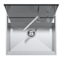
extra thick AISI 316 stainless steel bowl with radius "0" 54x34x18.3 h cm bowl balanced, removable, AISI 316 stainless steel cover with manual opening equipment: 3" ½, basket strainer waste, B overflow, Thalas telescopic mixer tap with remote control 1RUBTH tap hole: 2 standard holes 60 cm base unit for bowl 56x49 cm cut out flush: see technical sheet
