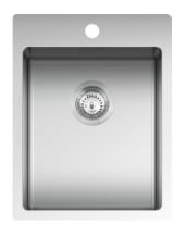
extra thick stainless steel AISI 304 bowl with radius "15" 34x40x19.5 h cm bowl equipment: 3"%, basket strainer waste, overflow with perimeter overflow tap hole 45 cm base unit for bowl 37x49 cm cut out flush: see technical sheet
